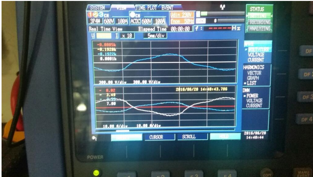
Figure 7 – Sawafuji waveform under load
