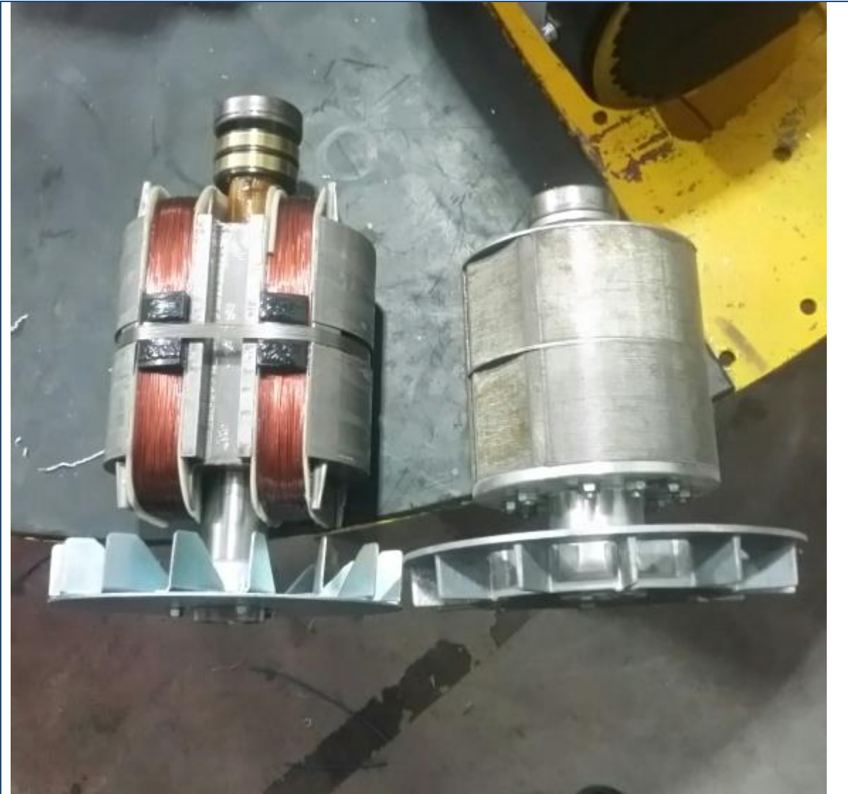
Figure 5 – Rotor Comparison (Sawafuji Left, RFL Alternator Right)
